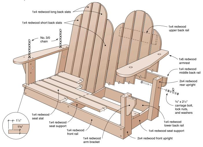
**2. Seat supports** The 1x4 seat supports are specially shaped to create the comfortable contoured seat and slanted back. Refer to the seat-support pattern (shown below) for specific details. Note that the back end of each seat support is miter-cut to a 15° angle and a portion of the upper edge is trimmed away to accommodate the five 1x4 seat slats.
