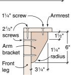
Set each armrest in position on the frame, with its wide front end on top of the front upright and its narrow back end on the rear upright. Attach each armrest with four  $2\frac{1}{2}$ -inch screws, driven into the uprights. Use one  $1\frac{1}{4}$ -inch screw to attach the armrest to the arm bracket.
