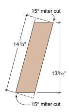
and mark the 15° cut. Next, using the pattern as a guide, mark the cut line through the squares in the grid. Cut along the segmented line with a sabre saw and lightly sand the edges smooth. Now, use this support as a template to mark the remaining two. That will ensure that all three supports will be identical.
