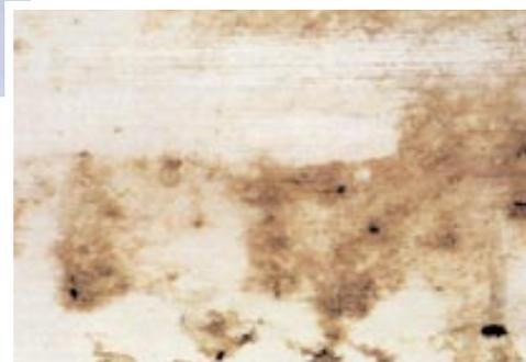
ferrocyanide, the presence of iron can be confirmed by a resulting blue color. If this test is negative (and the bleach test is negative), the discoloration present is likely the result of water soluble extractives. In most cases, this diagnosis can be confirmed if the discoloration can be removed by an application of oxalic acid.
