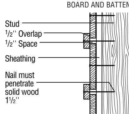
Use one nail, an inch from the lap, for 6-inch channel shiplap. Face nail with two nails per bearing for patterns 8 inches and wider. Space nails 1 1/2 inches from the edge of the overlap and 2 inches from the edge of the underlap. Nail other widths proportionately. Position material to allow expansion clearance of 1/8 inch. Boards should be nailed to horizontal blocking installed between studs at no more than 24 inches on center.
