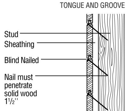
Face nail with two siding nails per bearing for patterns wider than six inches. Position nails one-quarter the width of the material from each edge. For narrower courses, one nail per bearing is enough—with the nailing point one inch from the overlapping edge.
