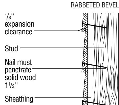
Face nail with one nail only per bearing. Drive nail so shank clears the top of the preceding undercourse.
